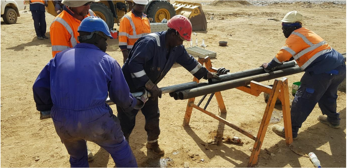
Fig 11.3. Recovering of a core from core barrel.
