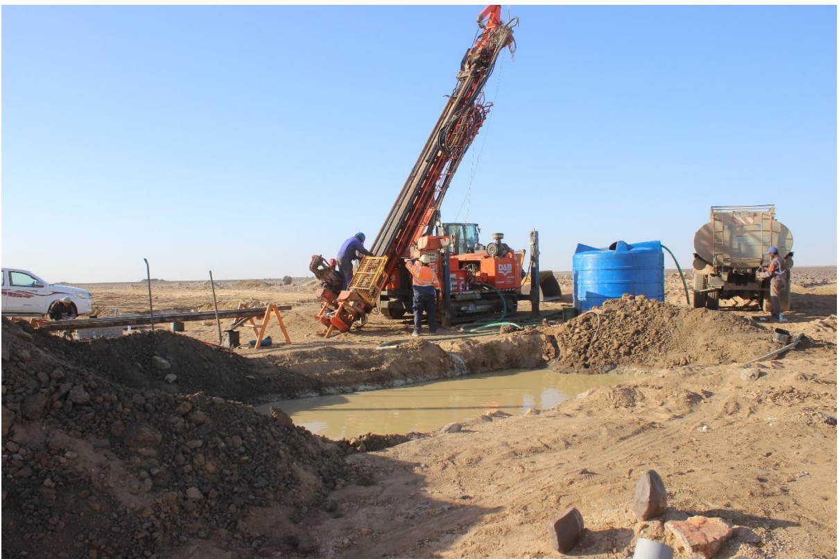
Fig 11.2. Drilling of DMDH-002a diamond hole, Azimuth 65 degree, inclination 55 degree
