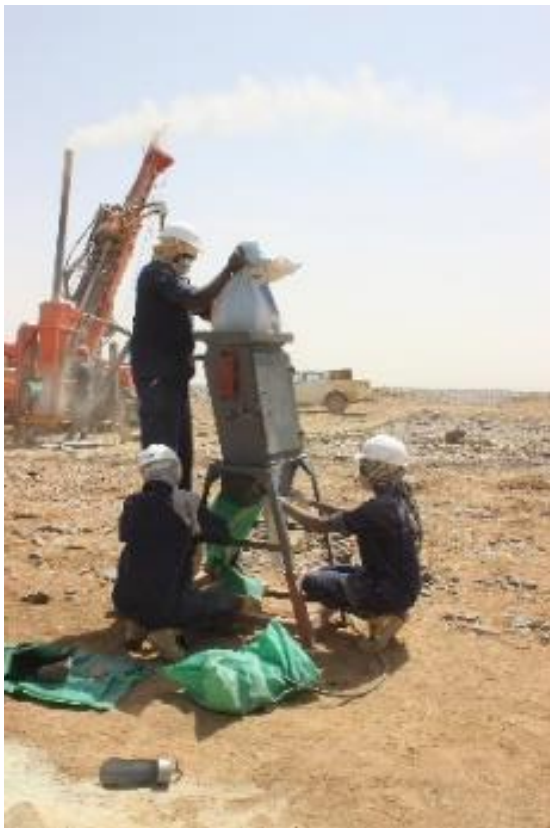
Fig 10.3. Splitting of the initial RC sample using a riffle splitter.
