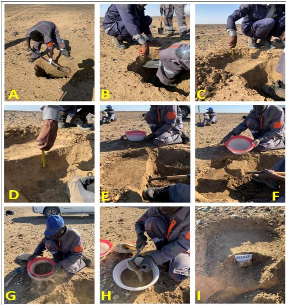
Fig 5.1. Soil sampling technique for the new Ionic Leach method applied on DM project.
