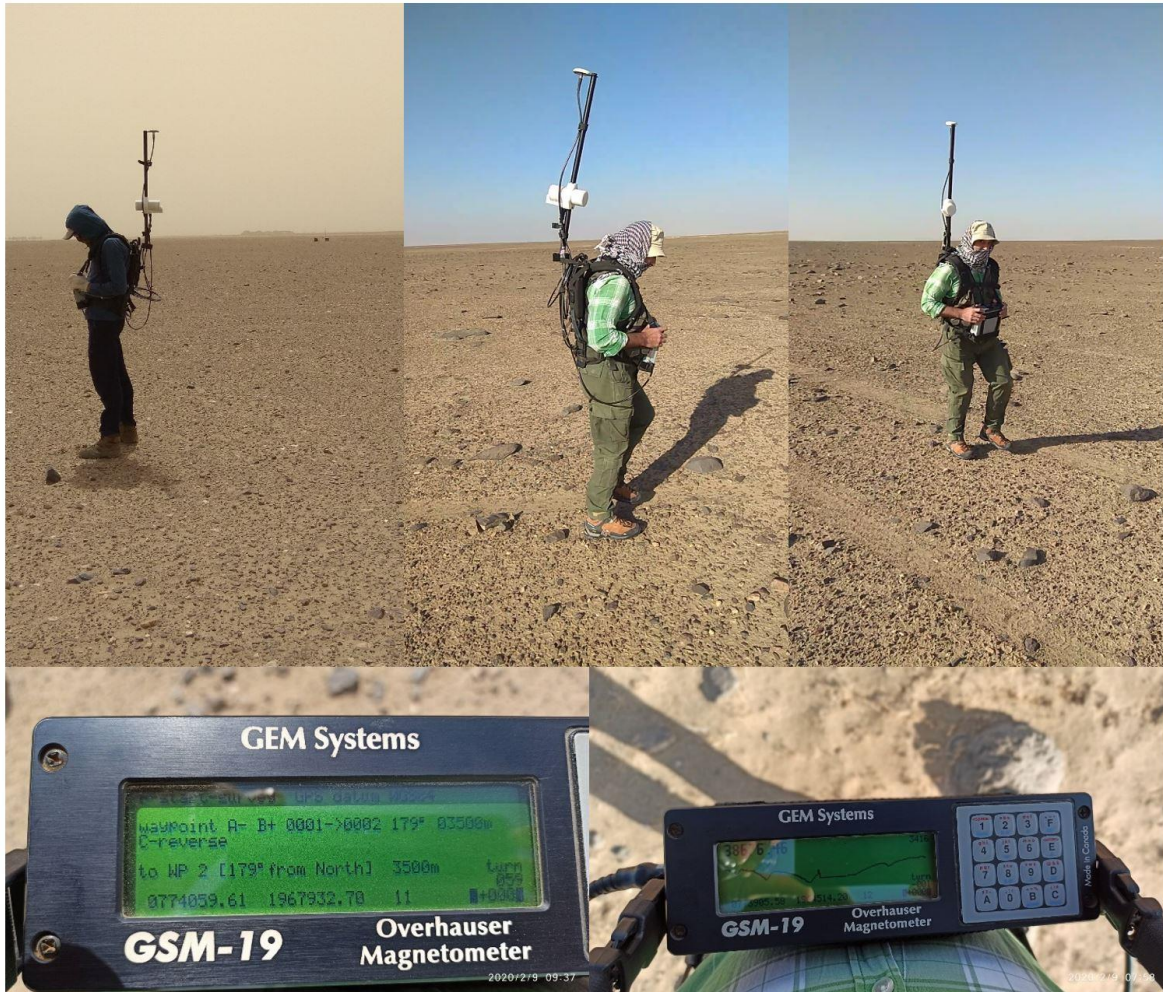
Fig 7.3. Surveyor equipped with GSM-19W magnetometer during the field work.
