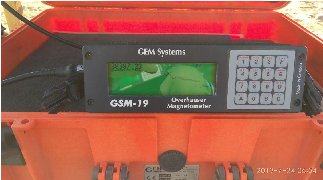
Fig 7.5. Variation curve of natural magnetic field on Base Station Magnetometer display.
