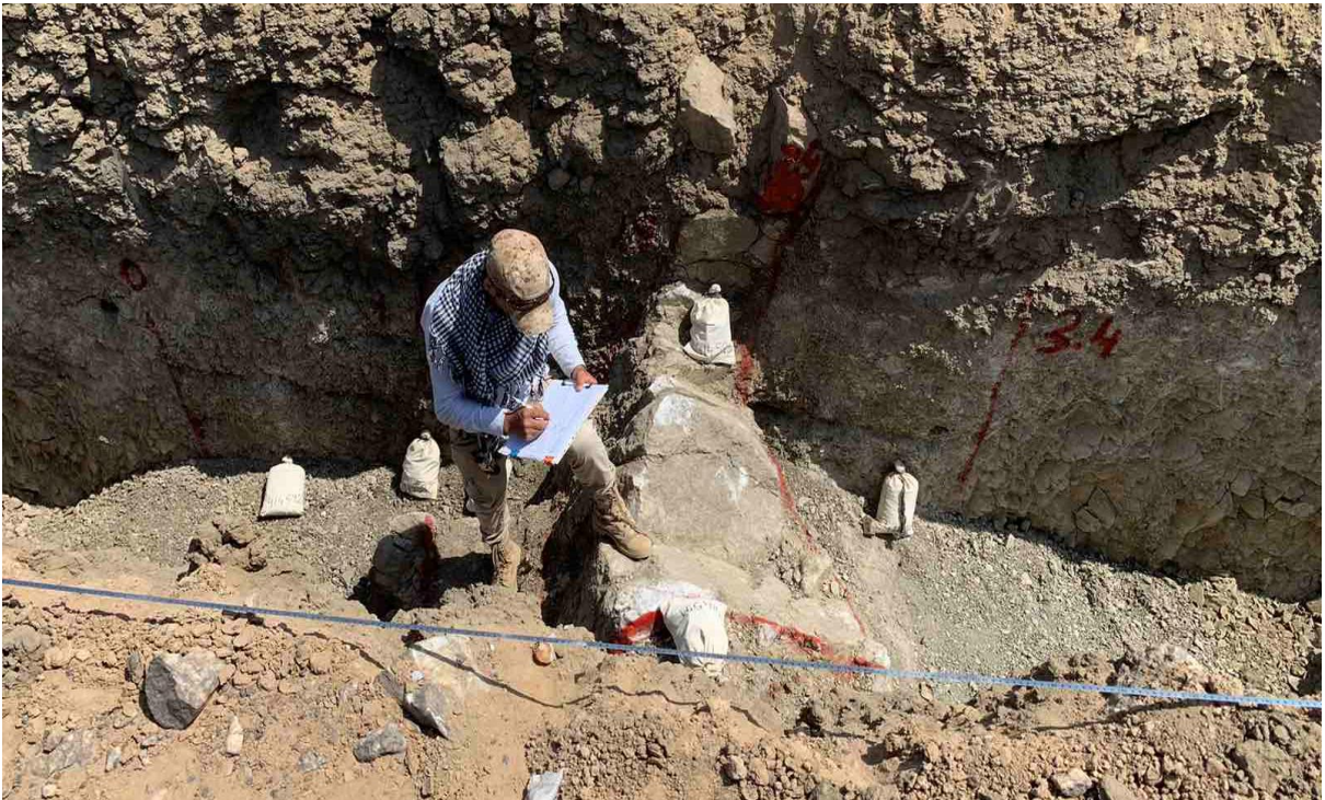
Fig 9.3. Trench logging and sketching by a geologist.
