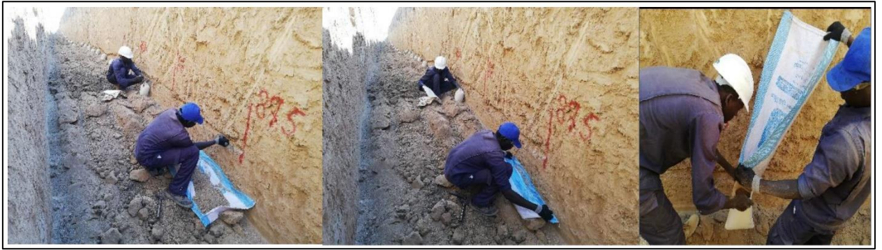
Fig 9.4. Channel sampling of shear zones stripped on trench wall. Chisel and hammer are used to cut channels.
