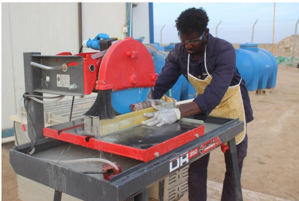
Fig 11.6. A core cutting procedure by a manual core saw.
