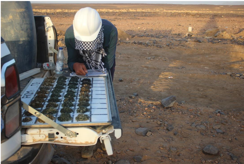
Fig 10.4. RC drill cutting logging by a geologist
