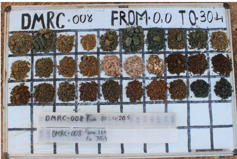
Fig 10.5. RC washed and screened drill cuttings on the logging desk. A quartz vein is exposed from 14m to 17m.
