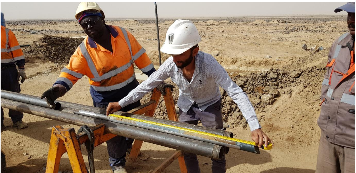
Fig 11.4. Measuring of the recovered core length.
